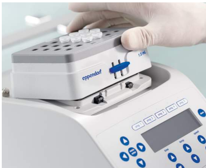
SmartBlock removal from Eppendorf ThermoMixer® C
